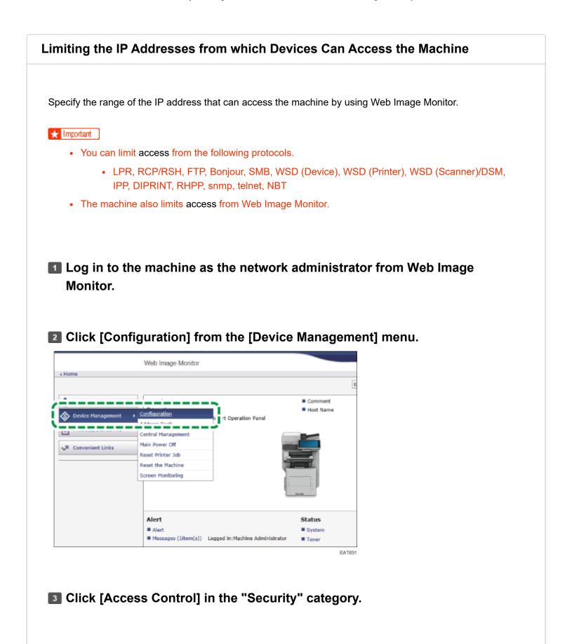
In "Access Control", click [Active] and specify the range of IP addresses that have access to the machine.
